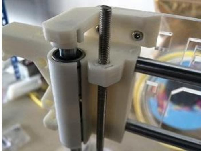
4. Attach the finished XZ plate to the chassis. The XZ plate should be sitting between the two fender washers on the chassis. Do not tighten the nuts yet.
