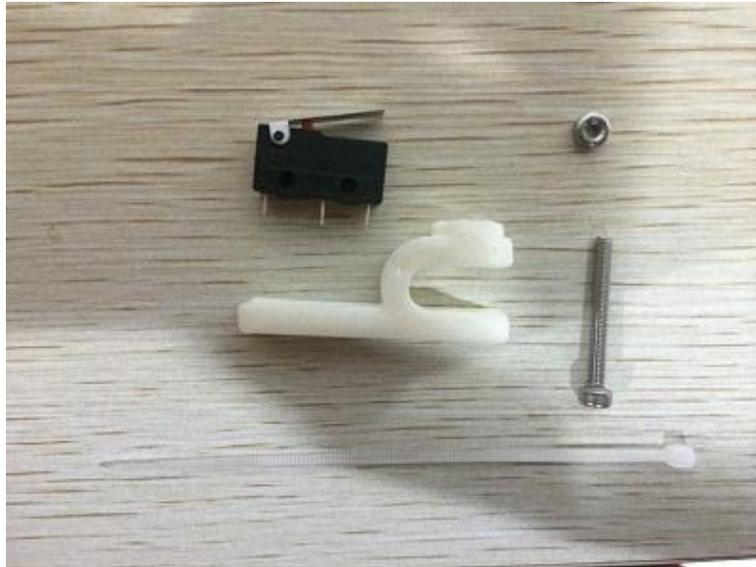
1. Attach the end stoppers to the end stopper mounts using zip ties. Wrap zip-ties around the two holes on the end stopper mount and the two holes on the end stopper.
