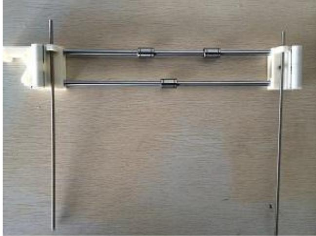
6. Attach the two 320mm 8mm precision rods through the LM8UU bearings.
