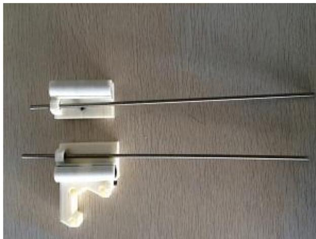
5. Attach the two 370mm 8mm precision rods with three LM8UU bearings.
