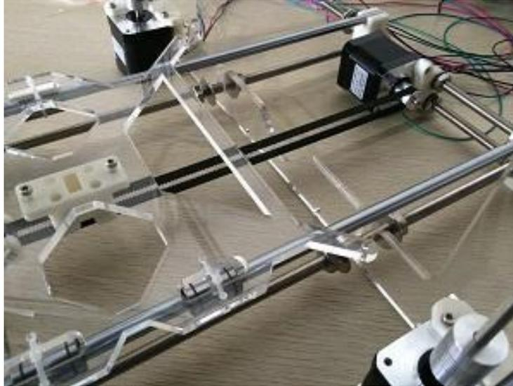
6.7 Attach the side panels to the main acrylic frame using three M3-25 and three M3 nuts on each side (first picture). Place the side panel with holes on the starboard side (the side with X motor). Place the bottom slot of the side panel between the fender washers on the longer rear threaded rod (second picture).
