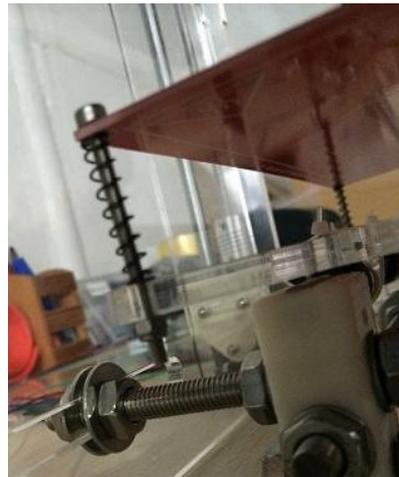
2. Attach the heatbed to the acrylic bed using m3-30 screws, springs, and m3 locking nuts. The order is: m3-25 screw – heatbed – spring- acrylic bed – m3 locking nut. Repeat this for all four corners.
