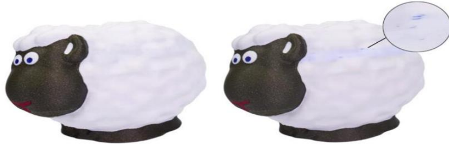
The sheep on the right has the white color contaminated by the blue pigment from the previous filament
