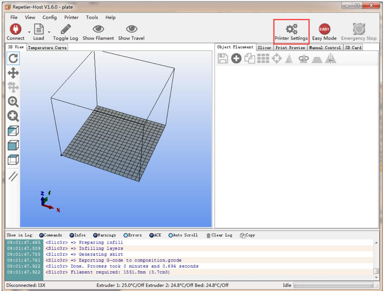
Select corresponding COM port of the printer and baud rate as 250,000 in the drop-down menu. Click Apply after the setting. Shown as below.
