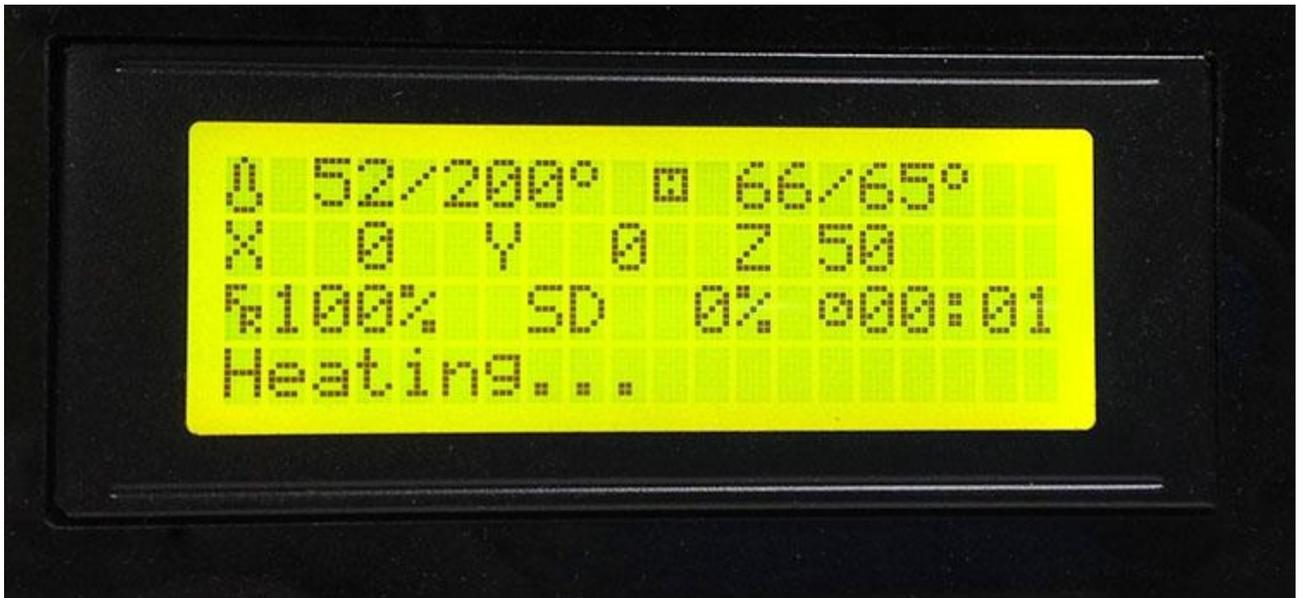
When heating is completed, it begins printing automatically.
