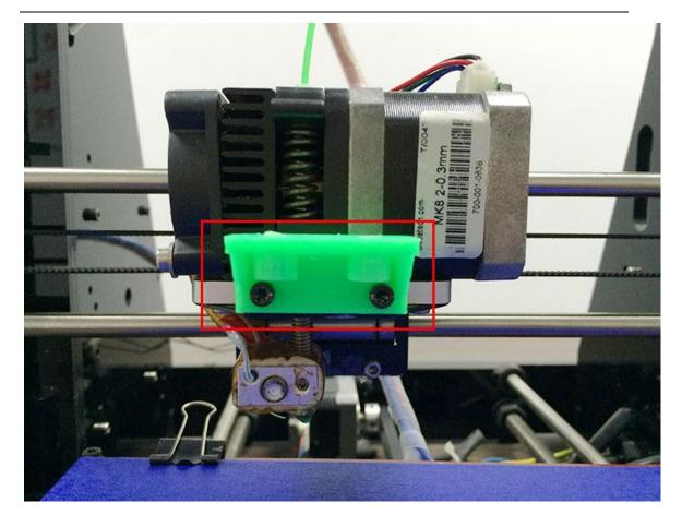
3. Fix the 3DTouch sensor on the sensor mount with 2 M3\*16mm screws and 2 M3 nuts.
