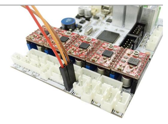
Connect the 2 pin wire to the Z min pin.
