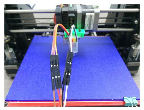
**Step3**. Connect the extended wire to the GT2560 control board.
