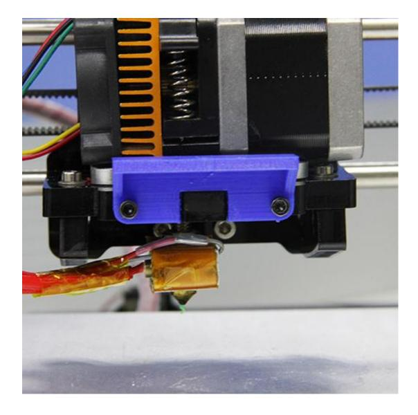
3. Fix the 3DTouch sensor on the sensor mount with 2 M3\*16mm screws and 2 M3 nuts.
