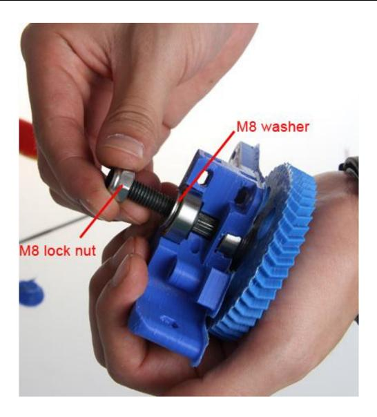
Add several(1 or 2) M8 washers, then mount the M8 lock nut by pliers or screw key.
