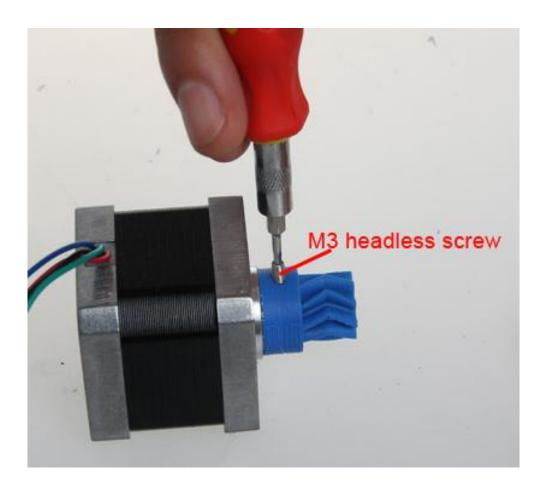
Use the M3 headless screw to fix the Small drive gear.
