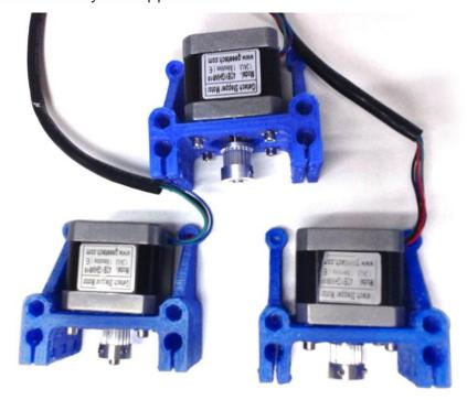
Fix motor to support with  $4 \times M3*10$  screw  $+ 4 \times M3$  washer; then Assemble deep groove ball bearing onto motor spindle, and fix it with  $2 \times M3*6$  set screw.
