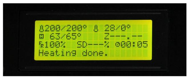
When heating is completed, it begins printing automatically.
