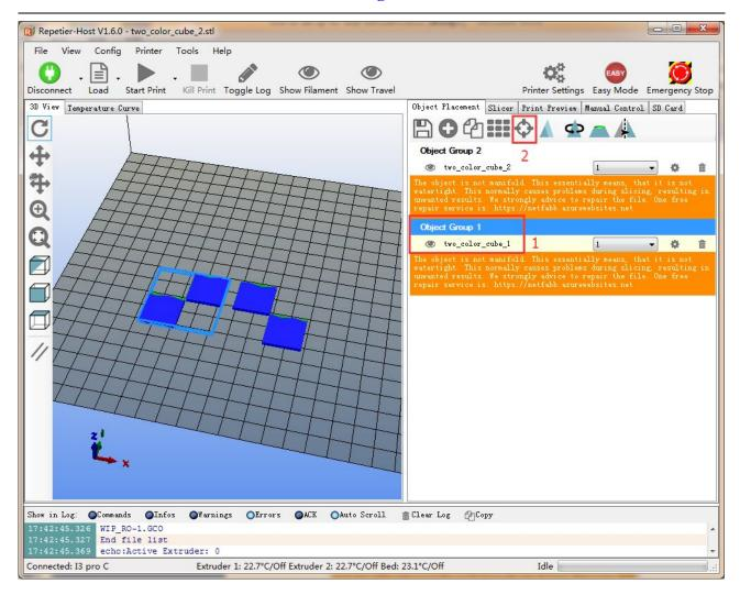
The object is now in the center of the hotbed. Put object 2 in the center of hotbed in the same way. After the setting, what you will see is shown as below:
