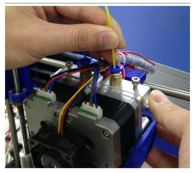
After pushing the filament into the bottom of hotend, use the feeding button on Repetier (as shown in following picture) to do manual feeding. If the nozzle can extrude filament fluently, the extruder is working well. If not, please refer to FAQ.
