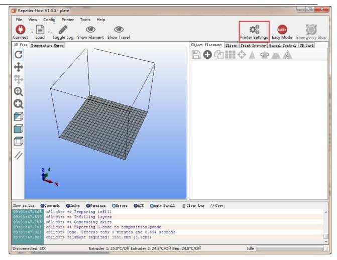
Select corresponding COM port of the printer and baud rate as 250,000 in the drop-down menu. Click Apply after the setting. Shown as below.
