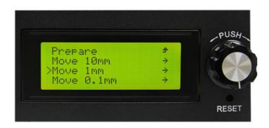
Choose the axis you need to move: Move X/Y/Z/E. Rotating the knob can make each axis move.
