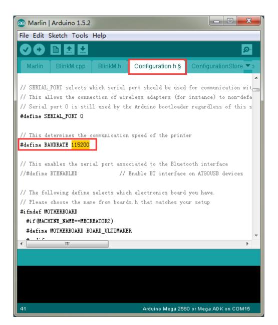
After successfully modifying the baud rate in firmware, change the baud rate in Repetier-Host to 115200 as well.
