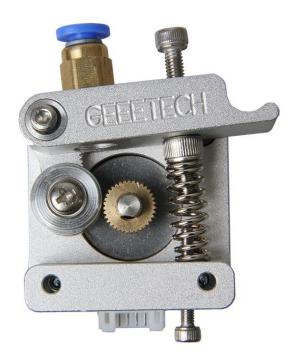
So far we have finished the feeder for a short distance MK8 Extruder.
