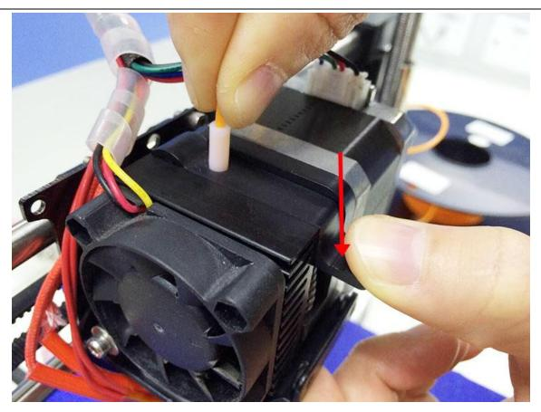
After pushing the filament into the bottom of hotend, use the feeding button on Repetier (as shown in following picture) to do manual feeding. If the nozzle can extrude filament fluently, the extruder is working well. If not, please refer to  $\underline{FAQ}$ .
