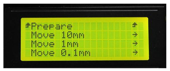
Choose the axis that you want to move by using Move X/Y/Z options. Turning the knob can make each axis move left and right or back and forth.
