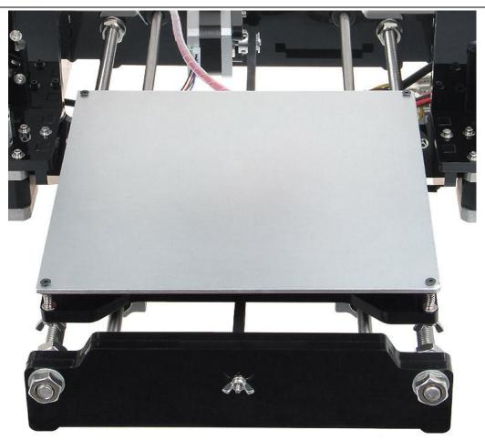
After finishing the adjustment of four corners, the entire leveling process is done. You can also move the extruder to the center of hotbed to verify leveling outcome.
