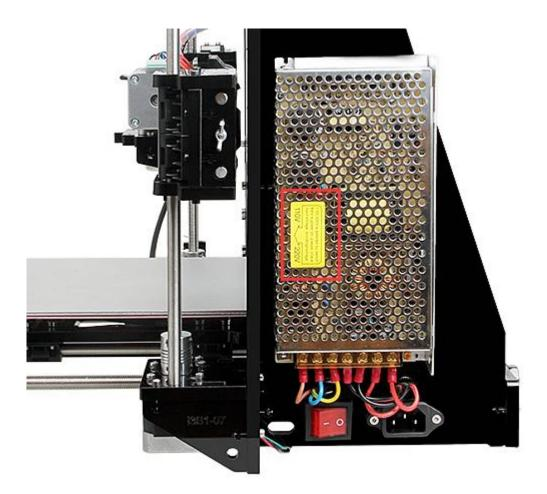
Check the power input of the power supply unit. You can choose either 110V or 220V according to the Power regulation in your country.
