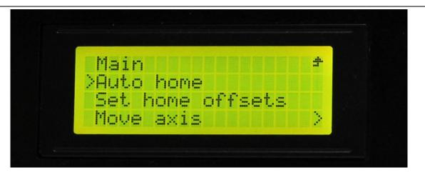
If you want to manually move the motor, you can unlock the motor. Unlocking method: Prepare>Disable steppers:
