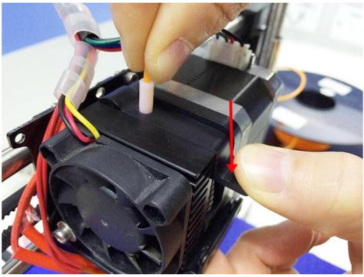
After pushing the filament into the bottom of hotend, use the feeding button on Repetier (as shown in following picture) to do manual feeding. If the nozzle can extrude filament fluently, the extruder
