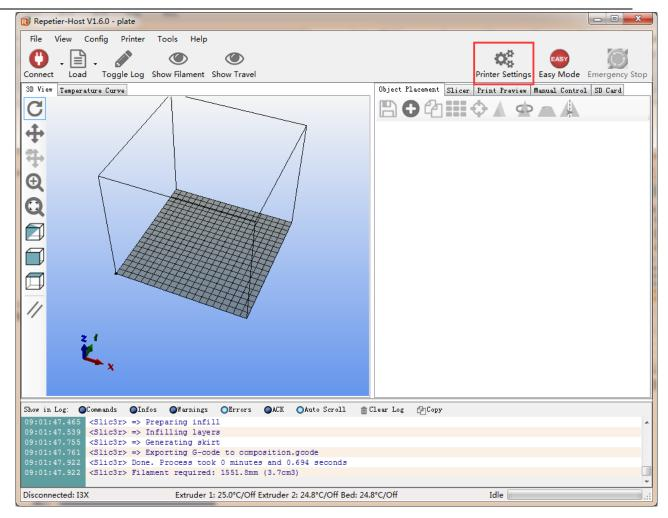
Select corresponding COM port of the printer and baud rate as 250,000 in the drop-down menu.
