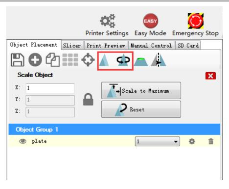
After the size setting, choose the slicing parameters which were imported previously in the drop-down menu, and click **slice with slic3r**.
