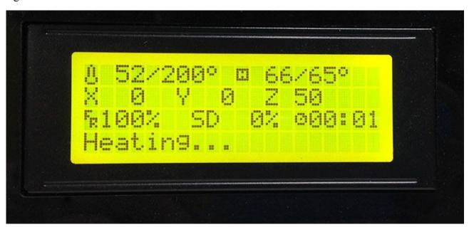
When heating is completed, it begins printing automatically.
