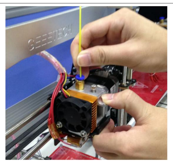
After pushing the filament into the bottom of hotend, use the feeding button on Repetier (as shown in following picture) to do manual feeding. If the nozzle can extrude filament fluently, the extruder is working well. If not, please refer to <u>FAQ</u>.
