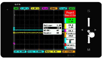
• In the Main Menu or Sub-menu interface, tap "<" >" Button or horizontally Slide "<">" to adjust the Menu parameters. (When you move positions in the Sub-menu interface, tap and hold your finger for continuous operation).
