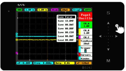
• When you turn on Auto Fit in Trigger, double-tap the non-button identification area, the device will automatically adjust the amplitude, the time base, and the trigger grid.
