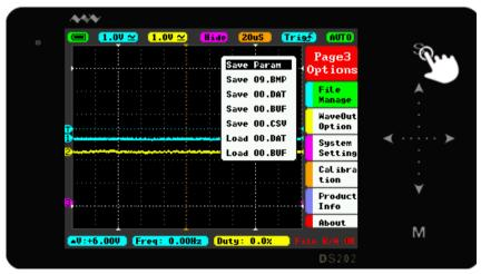
• In the Main Menu or Sub-menu interface, tap "A"" "or vertically Slide" A... "To select items upward or downward.
