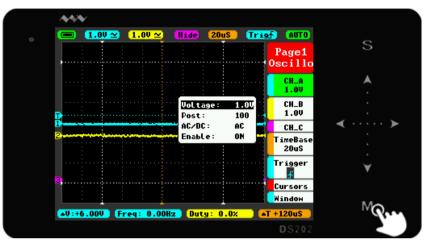
• In the Sub-menu interface, tap "S" Button to confirm the selection of operation.
