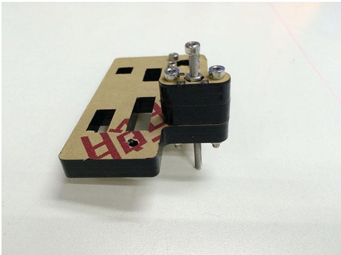
Step 3. Mount the endstop
