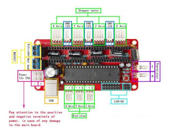
Note: there are two stepper motors for Z axis, the connecter is as shown in the following picture:
