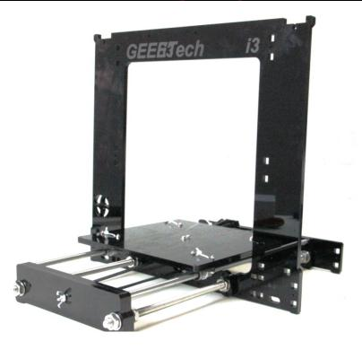
Step2. Screw up the main frame to the acrylic fender with M3 x 20 screws.
