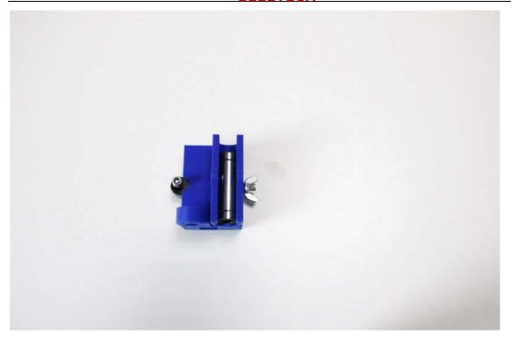
Step3. Insert another linear bearing into the slot of left end. Then lock the bearing with M3x 16 screw and nut. Do the same to the right end.
